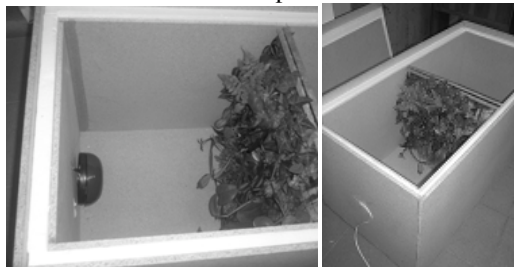
Figure 12: Box with sound level meter and green wall prototypes.
